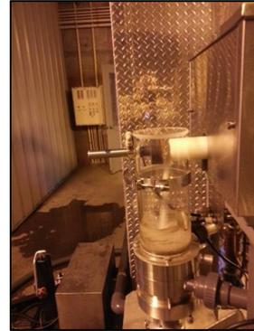
Polyblend® DP800 Dry Polymer Preparation System Demo Trailer
